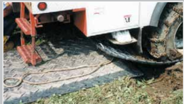
Driver called for help. AlturnaMATS® were brought to the scene and tied to the chains. By putting the vehicle in reverse, the MATS were drawn under the wheels. A second MAT was placed behind the wheels enabling the vehicle to back out easily.
