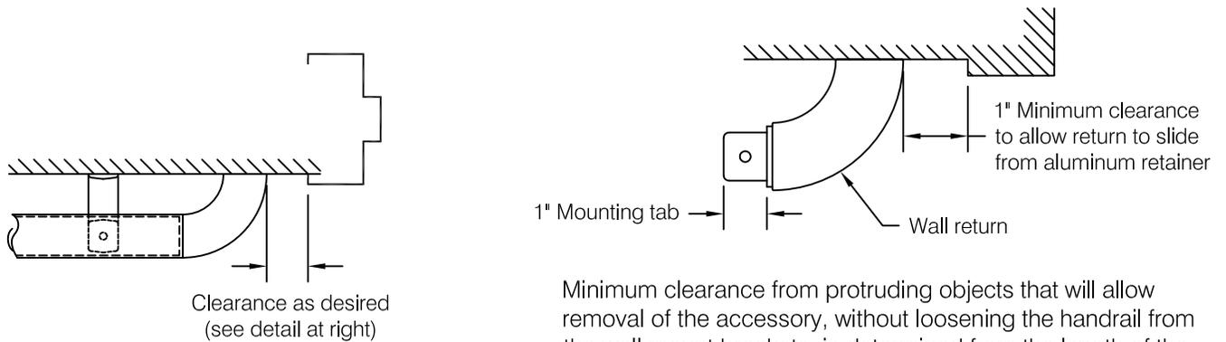
Minimum clearance from protruding objects that will allow removal of the accessory, without loosening the handrail from the wall mount brackets, is determined from the length of the mounting tab as shown.
